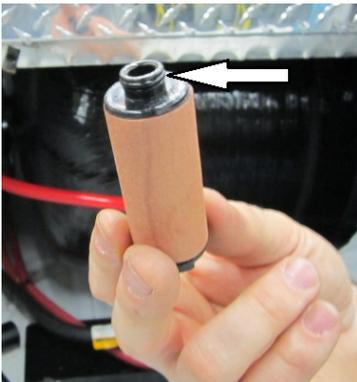
9. Using the filter socket, re-install filter housing and torque to 45 ft-lb.
