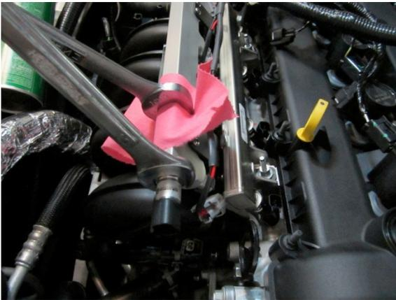
9. Fitting connecting low pressure hose to fuel rail, torque to 35 ft-lb.
