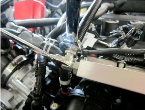
4. Locate filter housing and using the filter housing socket, loosen and unscrew the filter housing.
