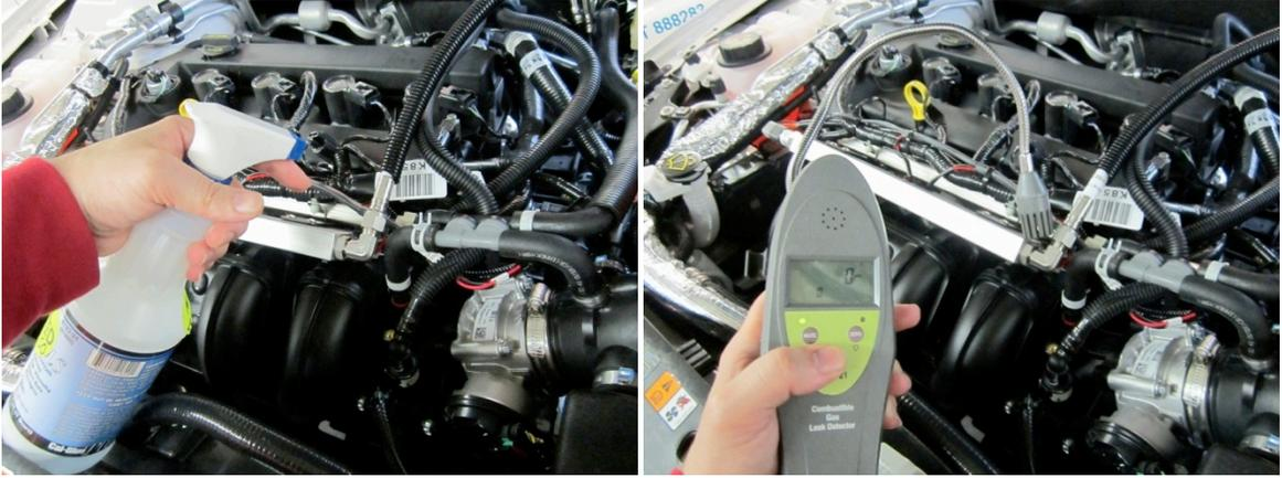
12. If there is a leak, add an additional  $\frac{1}{4}$  turn to the low pressure hose or high pressure hose connection(s). Perform another leak test. If leak persists, notify your supervisor for further instructions
