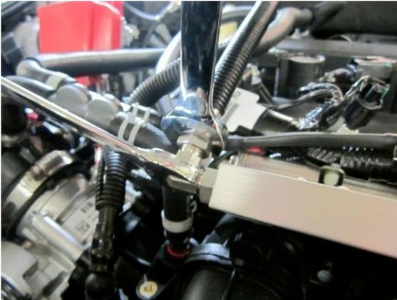
4. Disconnect and remove desired high pressure hose(s).
