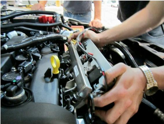
6. Hand start the fuel rail bolts, then tighten to Ford specification. Use caution to avoid cross threading.
