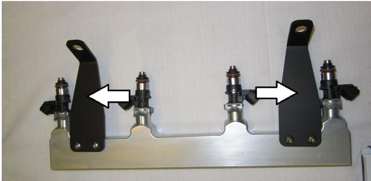
9. Plug in all injector connections, including interceptor harness or jumpers then nudge fuel rail evenly from side to side and ease it into place.
