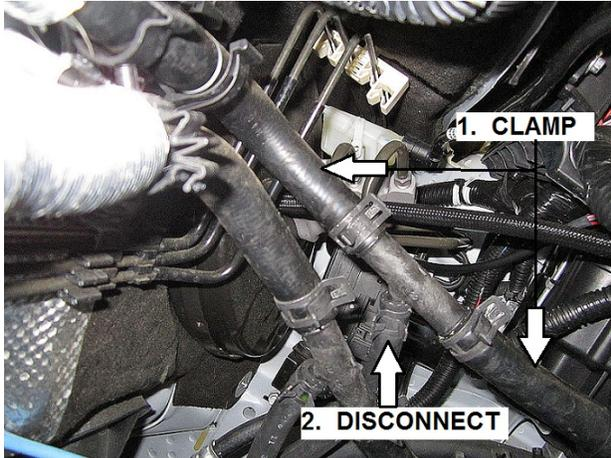
**Note:** there is coolant fluid still remaining in the kit lines. Drain the coolant hoses appropriately.
