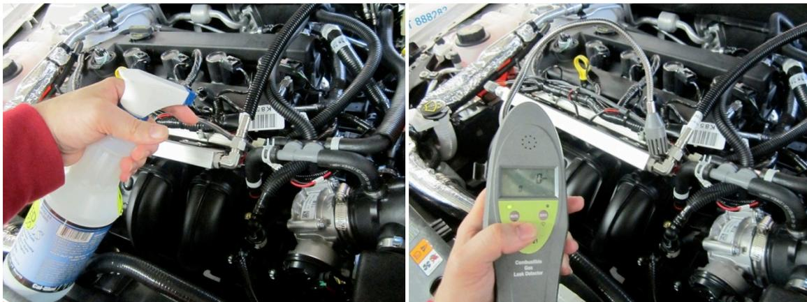
15. If there is a leak, add an additional  $\frac{1}{4}$  turn to the low pressure hose on the corresponding connection end. Perform another leak test. If leak persists, notify your supervisor for further instructions.
