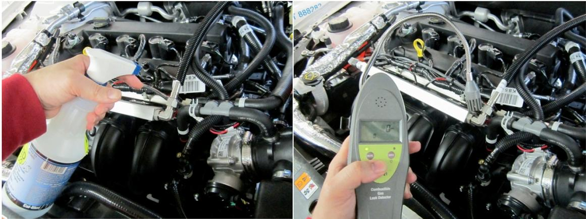
12. If there is a leak, add an additional  $\frac{1}{4}$  turn to the low pressure hose connection or transducer connection. Perform another leak test. If leak persists, notify your supervisor for further instructions
