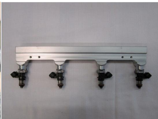
5. Assemble fuel rail with Injectors, fuel rail brackets (leave loose), and harness (bi-fuel system interceptor harness) or jumpers (dedicated system).
