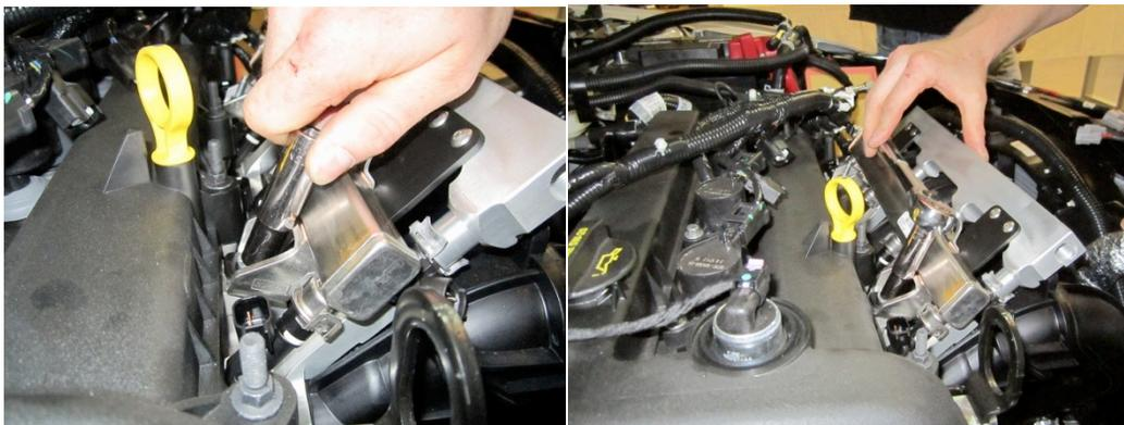
12. Tighten the fuel rail brackets using an Allen wrench.
