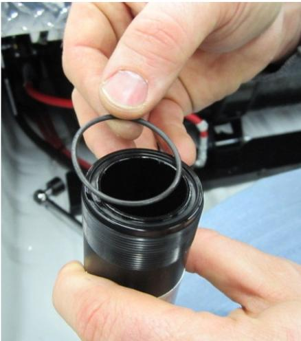
7. Install a new o-ring. Use parker lube and spread it generously over the new o-ring.
