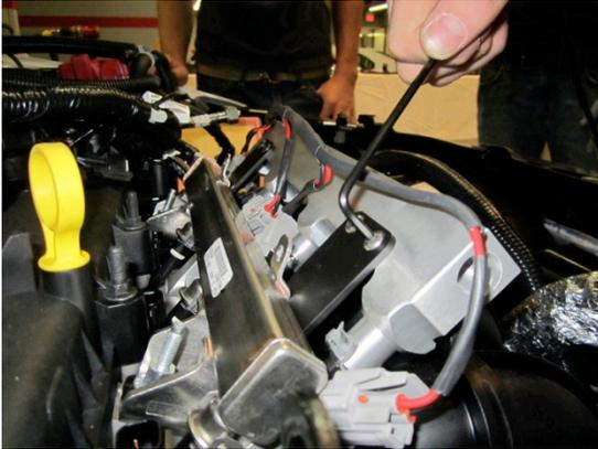
8. Low pressure sensor (Transducer) torque to 35 ft-lb.
