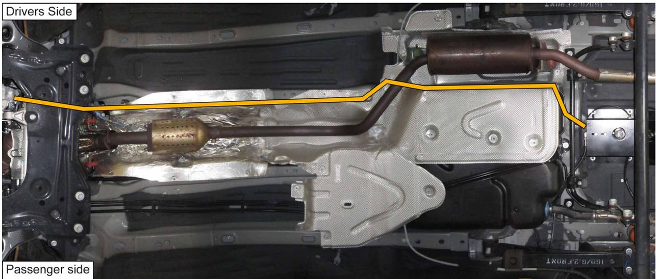
6. Re-attach the coolant hoses on both ends. Verify hose connections are attached to the corresponding direction of flow. IN to IN, OUT to OUT.
