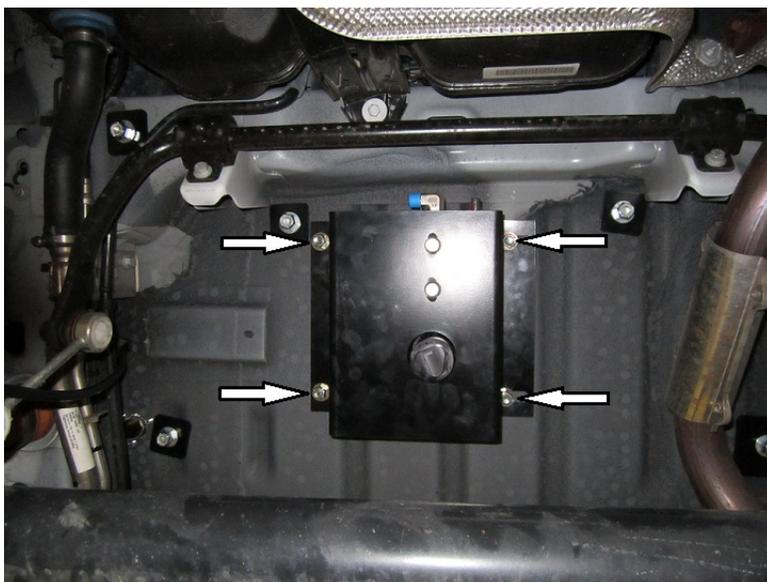
9. Attach the new regulator assembly. Ensure all labels are present. Reconnect all hoses and rear harness. Hand tighten low pressure hose then make a mark on the nut of the hose and make a full rotation plus  $\frac{1}{4}$ - $\frac{1}{2}$  turn. Torque the bolts holding the regulator to the vehicle to 40 ft-lb. Ensure to connect coolant hoses accordingly, IN to IN and OUT to OUT. Remove clamps and release the coolant flow. Tighten and torque fuel fill hose to 35 ft-lb.
