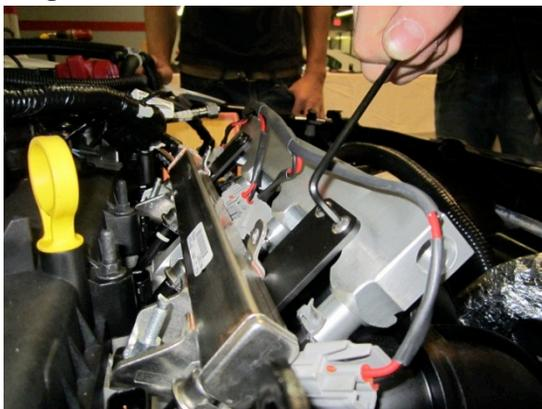
13. Once fuel rail has been secured, reconnect and tighten the low pressure hose. To tighten the low pressure hose, first hand tighten as much as possible, then make a mark and make a full rotation plus  $\frac{1}{4}$ - $\frac{1}{2}$ . When tightening, ensure you have a counter balance to avoid damaging the fitting, fuel rail, or threads.
