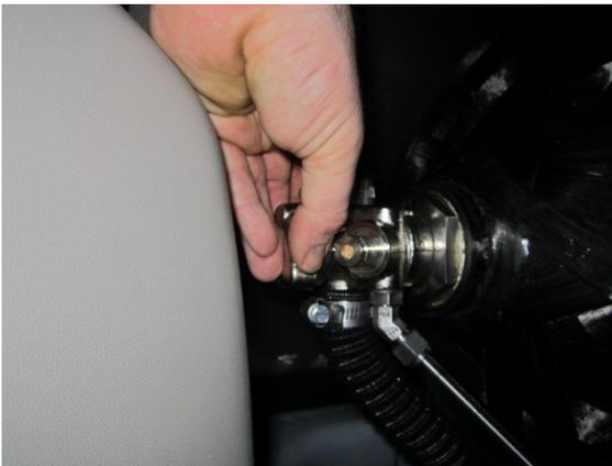
3. Clamp the OEM coolant hoses to restrict coolant flow. Work on one hose end at a time.
