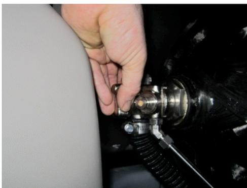
3. If vehicle is **operational** (does not apply to Bi-Fuel systems), depressurize the system by running the vehicle on CNG until the vehicle stalls. As an extra safety precaution, also crack the low pressure hose one half turn at a time to ensure all pressure has been vented. If the vehicle is **not operational**, crack and loosen the low pressure hose on the fuel rail side one half turn at a time until all pressure has been vented.
