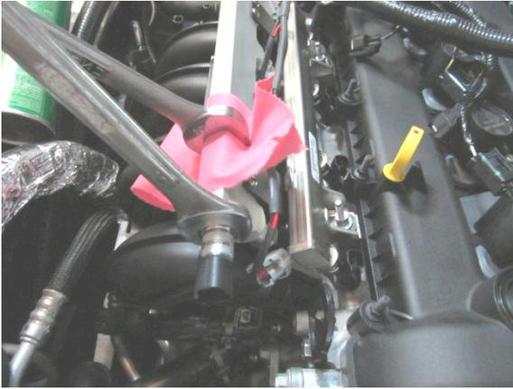
6. Re-tighten the low pressure hose. To tighten the low pressure hose, first hand tighten as much as possible, then make a mark and make a full rotation plus  $\frac{1}{4}$ - $\frac{1}{2}$ . When tightening, ensure you have a counter balance to avoid damaging the fitting, fuel rail, or threads.
