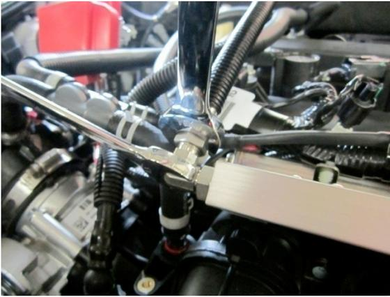
4. Disconnect the injectors from its jumper plugs or interceptor harness.
