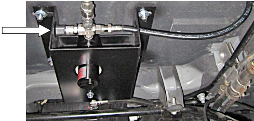
6. Verify the replacement transducer is rated for 5000psi. Replace transducer and tighten/torque to 35 ft-lb.
