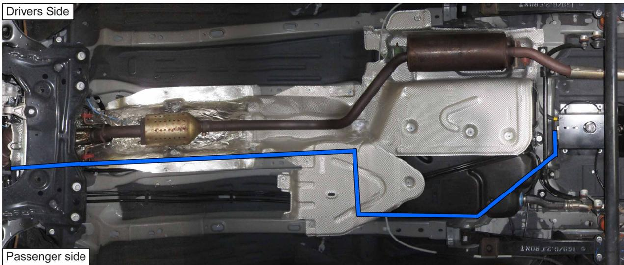
5. Install new hose and secure into place. Hand tighten both ends of the hose to their designated connection point and using a wrench tighten an additional  $\frac{1}{4}$ - $\frac{1}{2}$  turn. Verify warning labels are on both ends of the hose.
