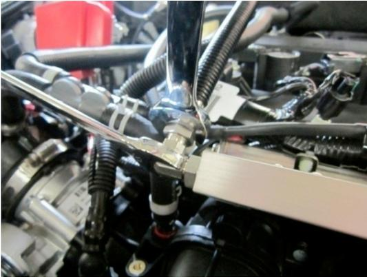
4. Upon fully releasing the pressure, loosen the fuel rail. Then:
