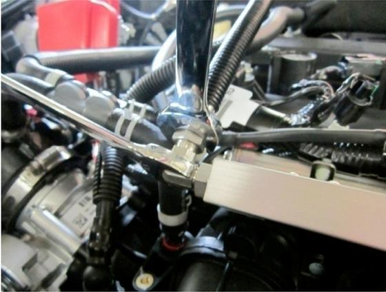
4. Remove the low pressure line by disconnecting it from the fuel rail and from the regulator and un-securing it from the undercarriage. The p-clamps and screws may be reused.
