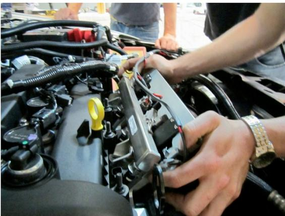
7. Remove the damaged injector(s).
